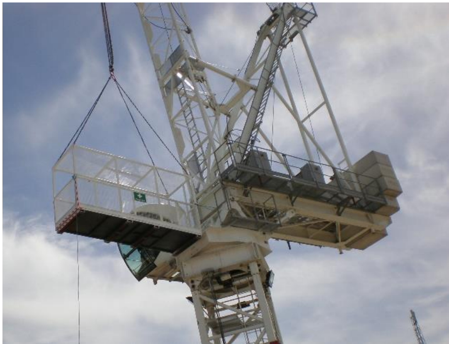
Figure 3: Example of a purpose-designed rescue man-riding carrier
