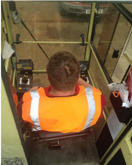
Figure 19: A narrow cab door makes access to the casualty difficult as they must be lifted over the seat
