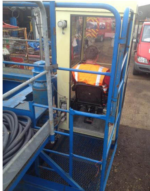
Figure 20: Small walkways also restrict access
